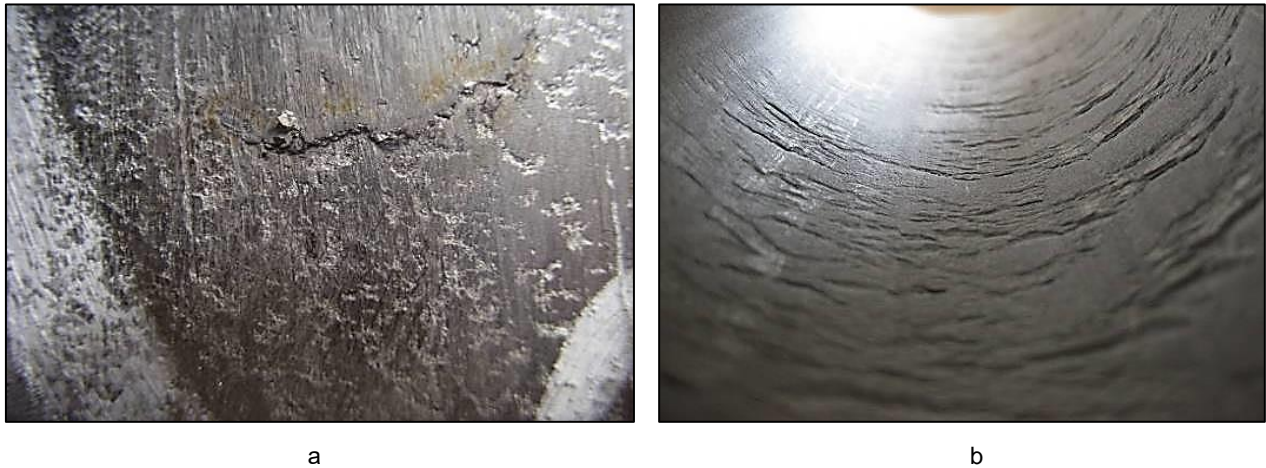
Figure 5. Appearance of defects (breaches in integrity) on the inner surface of the pipe: a – longitudinal cracks; b – rough 'ripples'.
