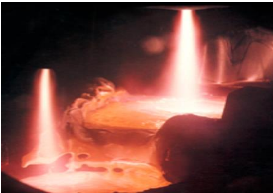
Fig. 7 – Operation of plasma torches of a plasma arc furnace [25]
