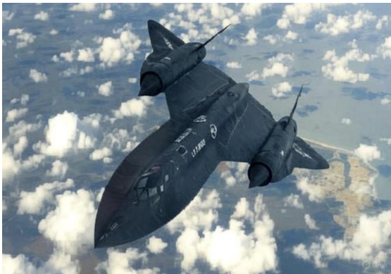
Fig. 3 – SR71 reconnaissance aircraft (first use of \beta -Ti alloys [5])
