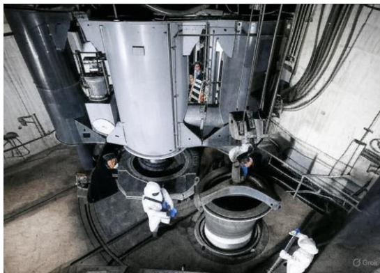
Fig. 5 – Vacuum arc furnace. Preparation for titanium melting [15]
