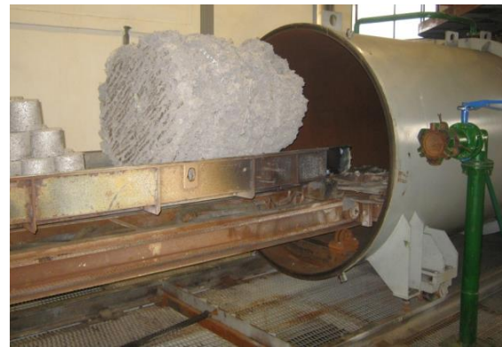
Fig. 6 – Electron beam furnace Zaporizhzhia Titanium-Magnesium Plant
