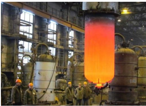
Fig. 1 – Chlorination of titanium. Zaporizhia Titanium-Magnesium Plant
