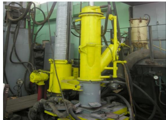
Fig. 8 – Laboratory chamber electroslag furnace
