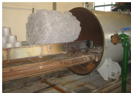
Fig. 6 – Electron beam furnace Zaporizhzhia Titanium-Magnesium Plant
