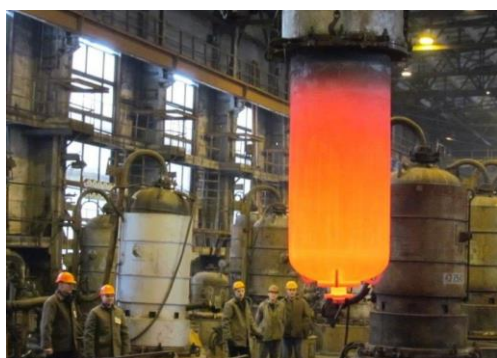
Fig. 1 – Chlorination of titanium. Zaporizhia Titanium-Magnesium Plant
