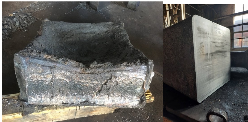
Fig. 5. Hot top cut 11% of 6,5 ton ingot 1.4541 (AISI321)
