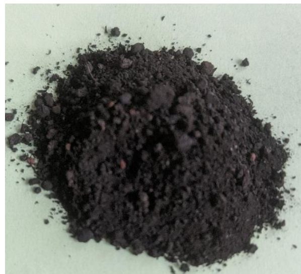
Fig. 1 – The appearance of "black lime" after carrying out compatible pyrolysis of components in the conditions of the spilled layer at temperature T_{max} = 1150^\circ\text{C} , \alpha_2 = 0.85 .
