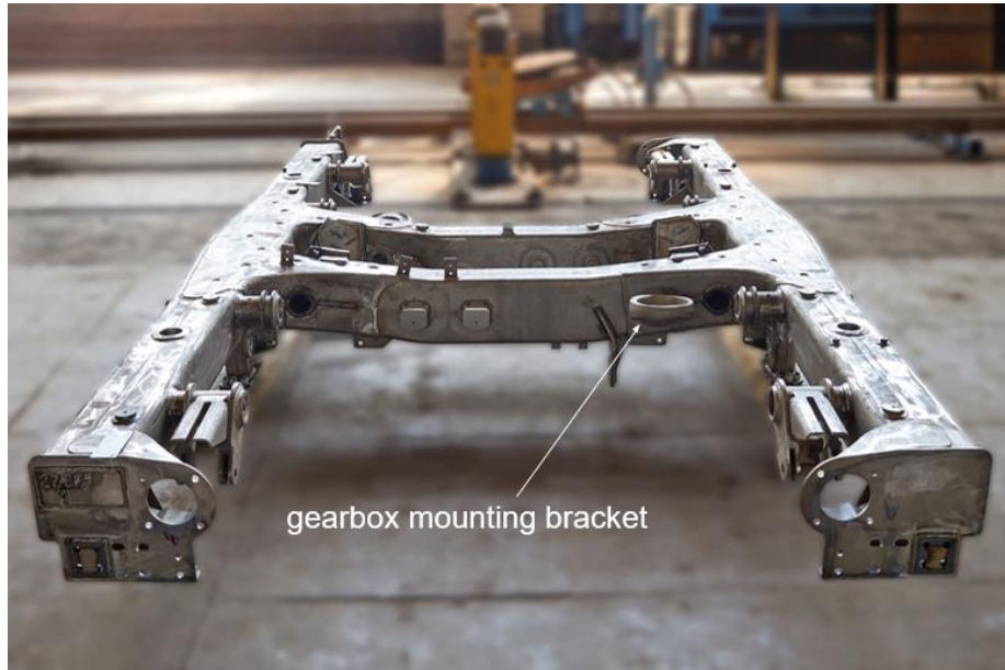
Fig. 1 – Bracket for mounting the gearbox of a 81-717 series carriage bogie.
