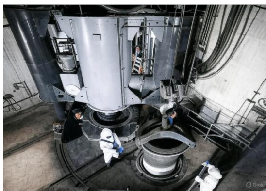
Fig. 5 – Vacuum arc furnace. Preparation for titanium melting [15]
