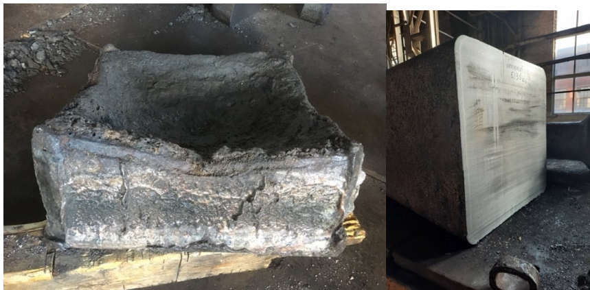
Fig. 5. Hot top cut 11% of 6,5 ton ingot 1.4541 (AISI321)
