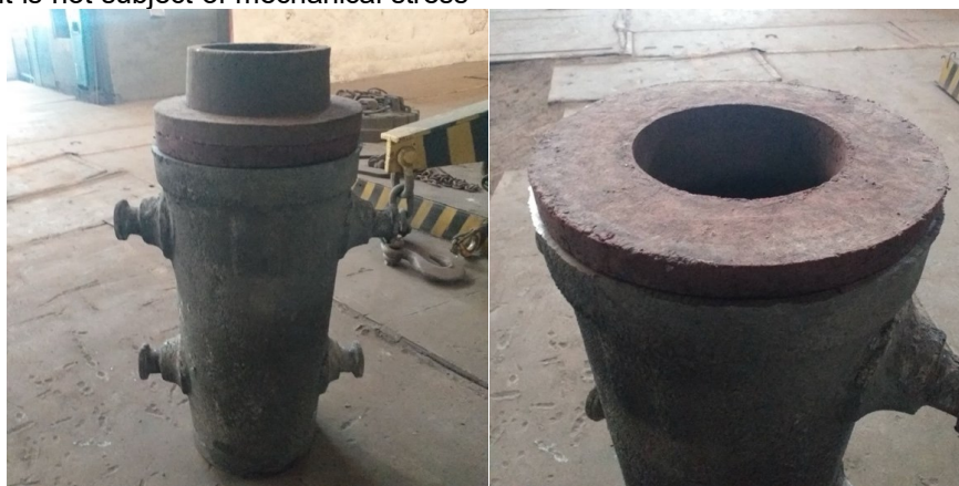
Fig. 12. Round-section mold (0,78 tn) with composite thermal insulation insert.
