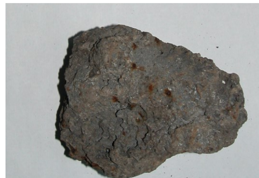
Figure 3. The appearance of bulk RSS in fraction 20-200 mm (a) and separate piece (b) - 85 mm in length.
