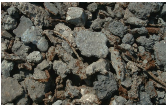
Figure 3. The appearance of bulk RSS in fraction 20-200 mm (a) and separate piece (b) - 85 mm in length.
